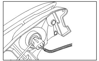
5. Disconnect the bulb base from the socket by lifting the plastic locking tab.
